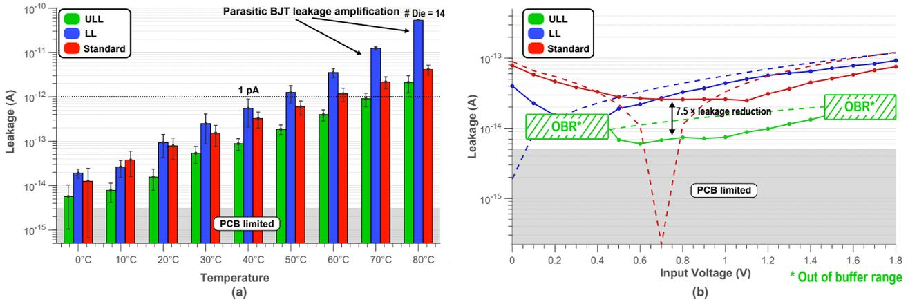
Fig. 5. (a) Measured maximum leakage between 0.5 – 1.5 V across temperature. (b) Measured (solid) and simulated (dashed) mean absolute leakage across the input voltage range at 20 °C.
