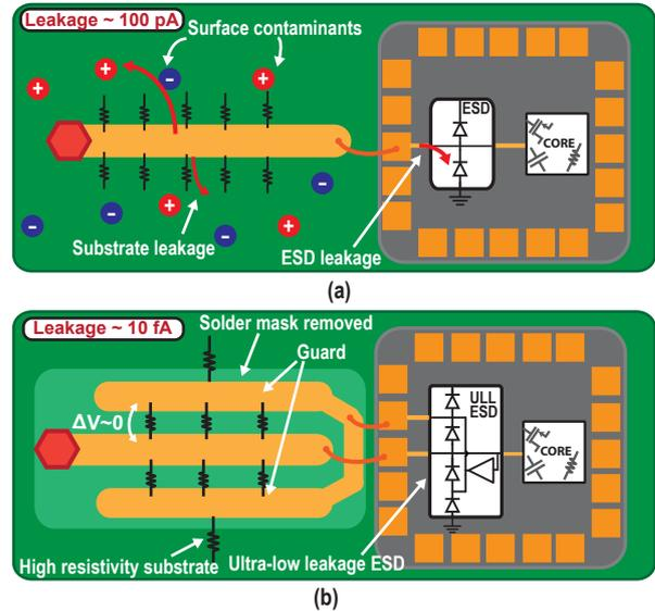
Fig. 1. Overview of leakage sources from: (a) Standard FR4 PCB and ESD; (b) Guarded low-leakage PCB and proposed ESD structure.
