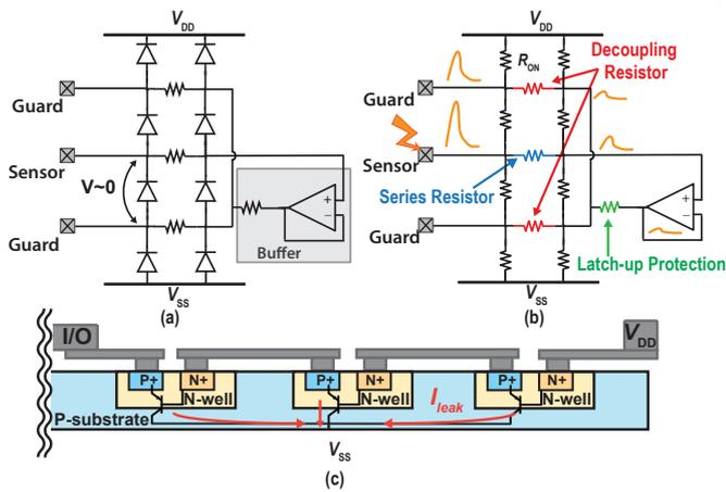
Fig. 3. ULL structure (a) schematic and (b) equivalent circuit during an ESD event. (c) Cross-section of a P-type diode stack illustrating parasitic BJT formed with the substrate.
