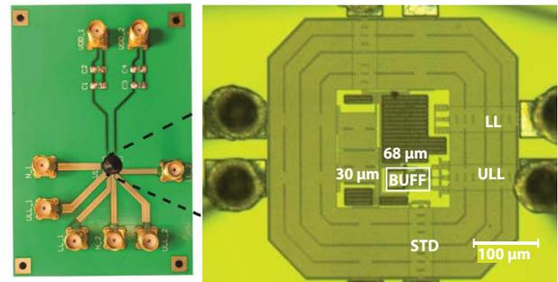
Fig. 4. PCB photograph and chip micrograph.
