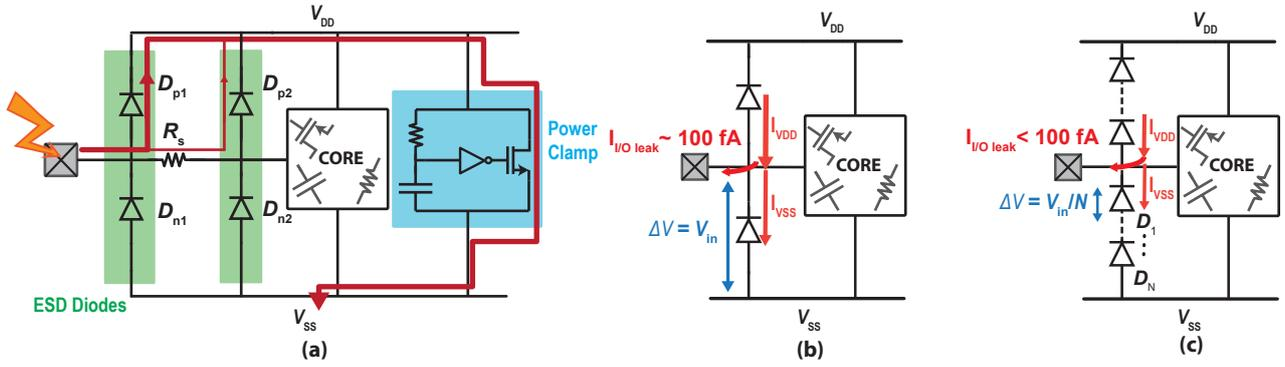
Fig. 2. (a) Standard whole-chip ESD protection during a positive charge ESD event. (b) Standard ESD leakage path. (c) Stacked diode leakage path.
