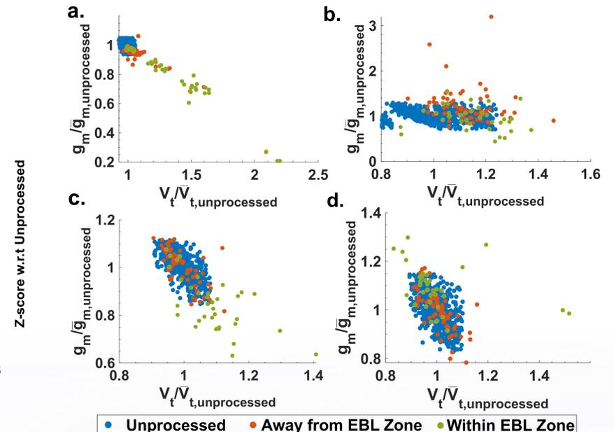
Normalized  $|V_t|$  and  $g_m$  after high-dosage treatment for a) PMOS I/O; b) PMOS core; c) NMOS I/O; d) NMOS core devices. Pixels within the e-beam blast zone (9 pixels around the e-beam site) are plotted with the pixels outside the zone and the unprocessed pixels
