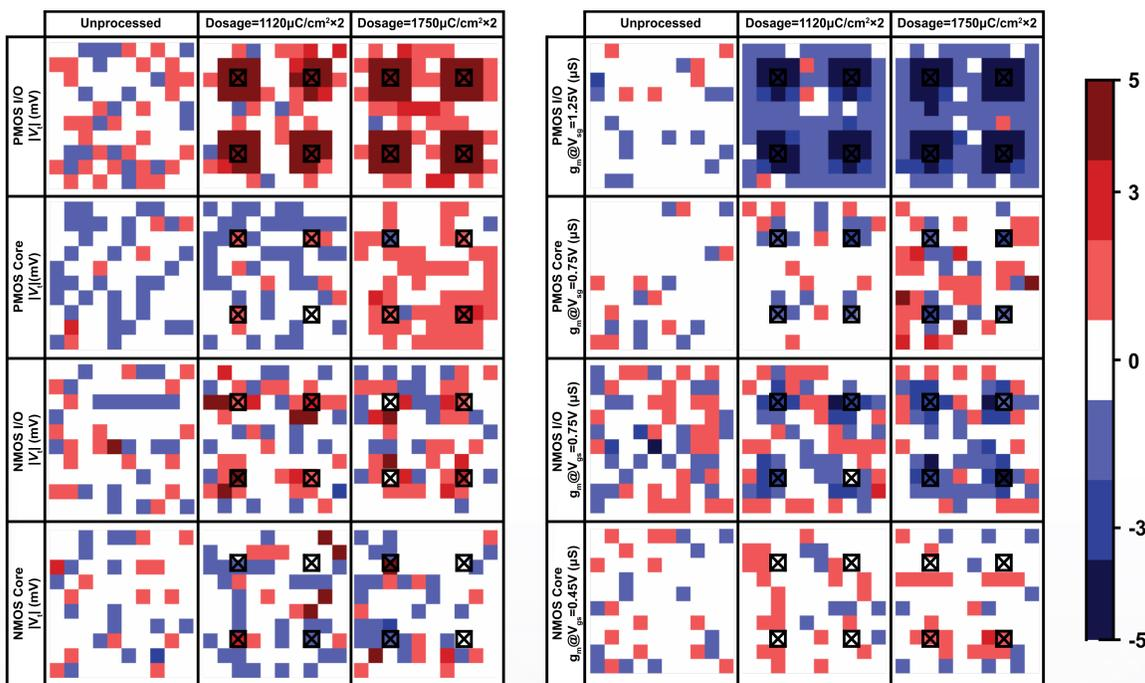
Measured Z-score of the extracted  $|V_t|$  and  $g_m$  shifts spatially plotted to correspond to the pixel array, with the four EBL sites marked.
