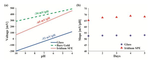
**Figure 6.** (**a**) Calibration curve of glass, bare gold SPE, and Iridium-Oxide electrode; (**b**) pH slope drift over several days for different electrode types.
