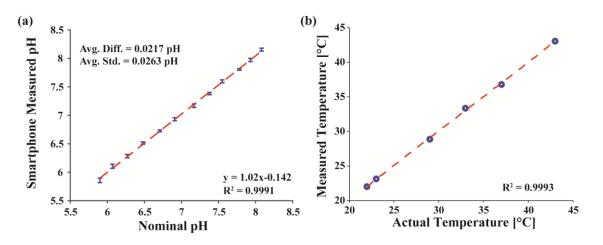
**Figure 5.** (a) Averaged measured pH data taken over one week (n = 7) for different nominal pH solutions ranging from 5.9 to 8.08 pH. The dotted line is a linear fit of the averaged data; (b) Temperature measured by the module compared to actual temperature recorded by a commercial thermometer from 20 to 45 °C.
