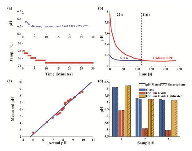
**Figure 7.** (**a**) pH and temperature settling over time of a fresh sputum sample; (**b**) Settling time of glass and Iridium Oxide electrode; (**c**) Sputum spiked to different pH levels measured with both glass and Iridium Oxide electrodes; (**d**) Actual sputum samples measured and calibrated.
