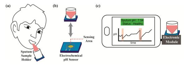
**Figure 1.** Overview of the smartphone-based pH sensor platform with (**a**) sputum collection via a sample holder, the bottom of which is (**b**) a reusable electrochemical pH sensor. (**c**) The entire holder attaches to an external electronic module that plugs directly into the headphone port of the smartphone to make and track measurements via a custom app.
