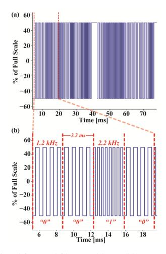
**Figure 3.** (**a**) A packet with frequency shift keying modulation and (**b**) a portion of the data decoded back to its original bits with zeros at 1.2 kHz and ones at 2.2 kHz.
