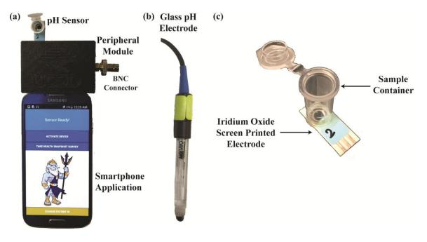
**Figure 4.** (a) Entire platform with the peripheral module inside a 3D-printed case, pH sensor chip, and smartphone running the custom CF application. Both (b) standard glass pH electrodes and (c) Iridium Oxide modified screen-printed electrodes can be used with this system.
