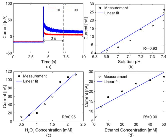
Fig. 6. Measured (a) transient waveforms, (b) pH transfer curve, (c) H<sub>2</sub>O<sub>2</sub> transfer curve, and (d) ethanol transfer curve.
