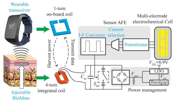
Fig. 1. Architecture of the injectable BioMote sensor.
