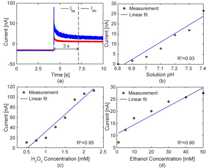
Fig. 6. Measured (a) transient waveforms, (b) pH transfer curve, (c)  $H_2O_2$  transfer curve, and (d) ethanol transfer curve.
