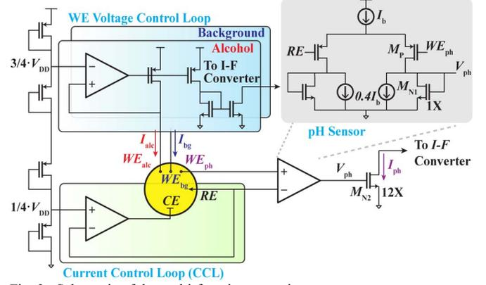
Fig. 3. Schematic of the multi-function potentiostat.
