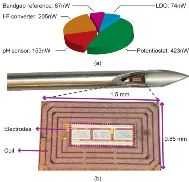
Fig. 7. (a) Simulated power breakdown and (b) annotated die photo.
