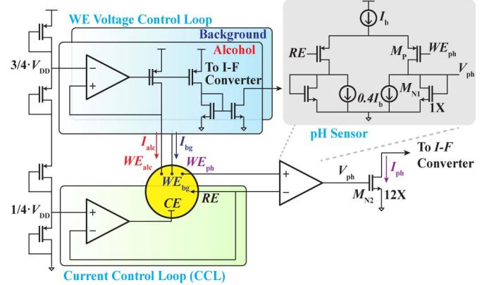
Fig. 3. Schematic of the multi-function potentiostat.
