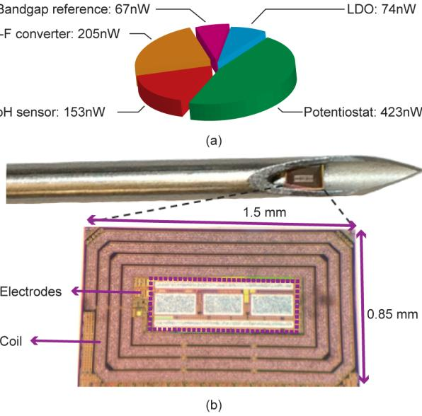
Fig. 7. (a) Simulated power breakdown and (b) annotated die photo.
