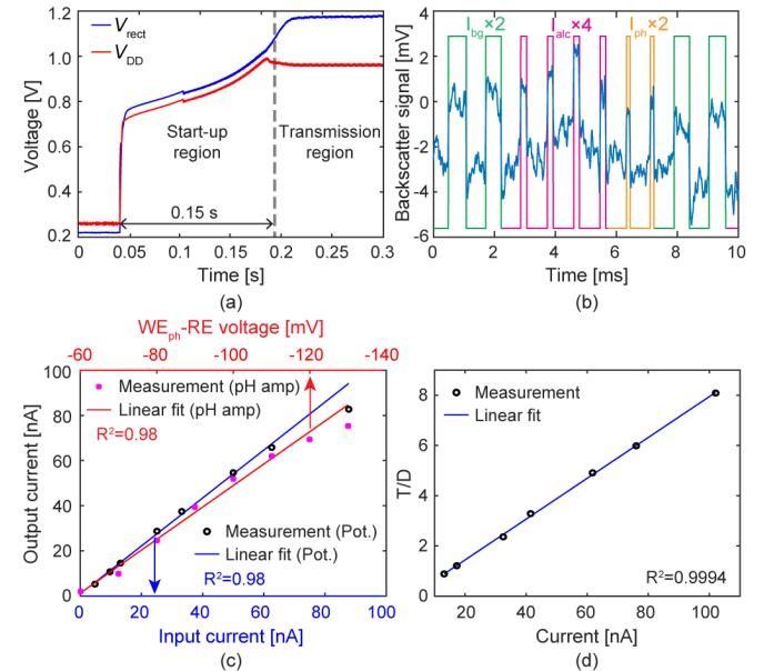
Fig. 5. Measured (a) transient voltage for wireless power transfer startup, (b) backscatter received output (blue) and  $I$ -to- $F$  converter output, (c) potentiostat transfer curve, and (d)  $I$ -to- $F$  converter transfer curve.
