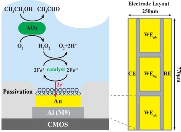
Fig. 2. (a) Illustration showing the alcohol assay and microelectrode layout, and (b) chronoamperometry measurement technique.
