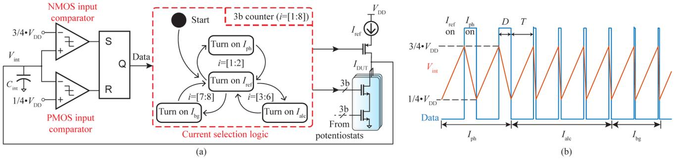
Fig. 4. (a) Schematic of the  $I$ -to- $F$  converter and current selection logic, and (b) timing diagram of the current selection logic.
