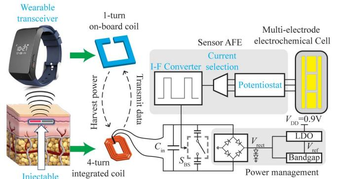
Fig. 1. Architecture of the injectable BioMote sensor.
