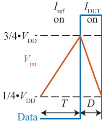
$$T = \frac{V_{DD} C_{int}}{2I_{ref}}$$
