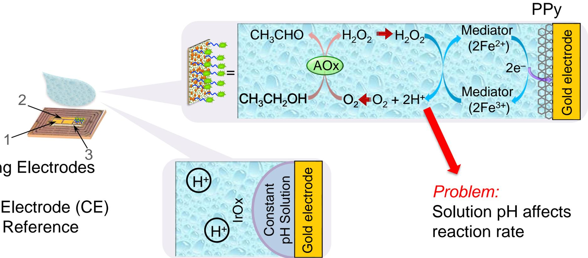
**Solution: Multi-electrode test cancels background signal and pH**
