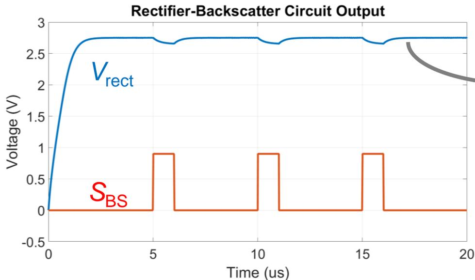
Small bypass capacitor → fast start-up, but large droops on supply
