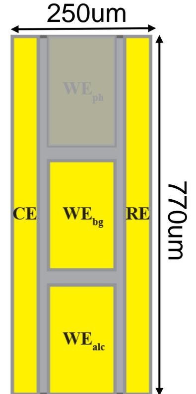
Low noise circuit (<3 nA) is required due to micro-electrodes
