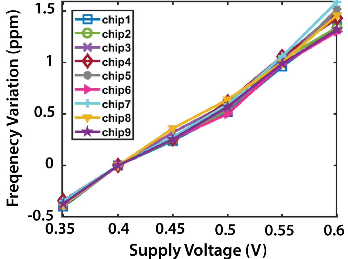
Temperature sensitivity < 25 ppm; Supply sensitivity < 2 ppm
