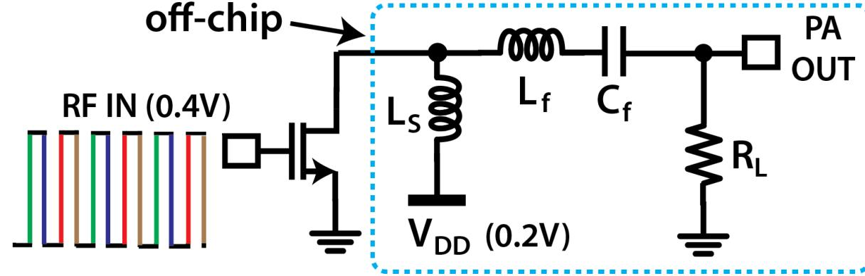
$$P_{out} = \frac{8}{\pi^2(\pi^2+4)} V_{DD}^2 / R_p = 0.058 V_{DD}^2 / R_p$$
