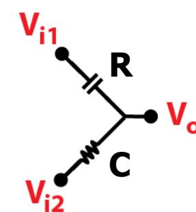
$$V_{o,ideal} = \frac{V_{i1}j + V_{i2}}{1 + j}$$
