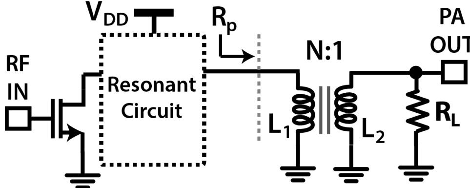
$$P_{\text{out}} \propto V_{\text{DD}}^2 / R_p$$
