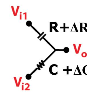
$$V_{o,\Delta RC} \cong V_{o,ideal} \frac{\Delta RC \cdot \omega + 2}{j \cdot (\Delta RC \cdot \omega + 1) + 1}$$
