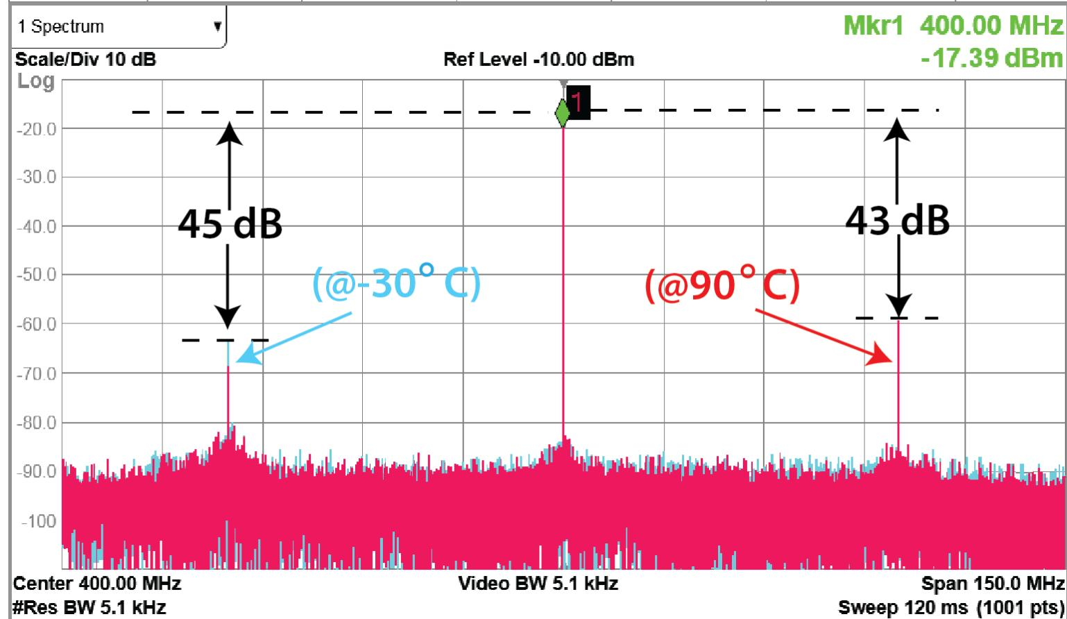
Carrier to spur ratio (CSR) > 40 dB across -30 to 90 °C
