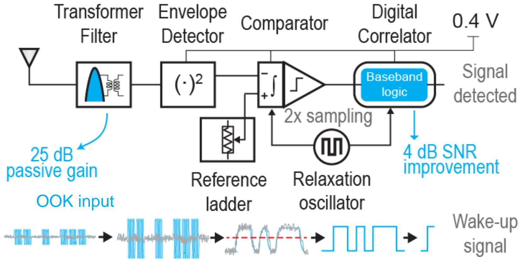
High  $R_{in}$  ED supports high passive gain front-end
