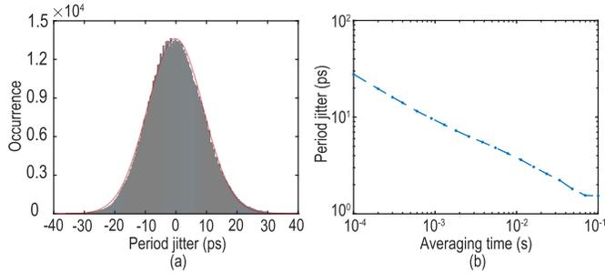
Fig. 13. Measured (a) FLL jitter histogram with 1 ms averaging and (b) jitter versus averaging time.
