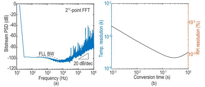
Fig. 14. Measured (a) TDC PSD and (b) temperature and RH resolutions versus  $T_{\text{conv}}$ .
