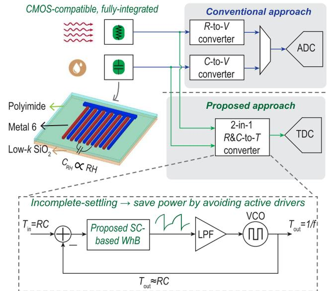
Fig. 1. Architecture of the 2-in-1 temperature and relative humidity sensor.
