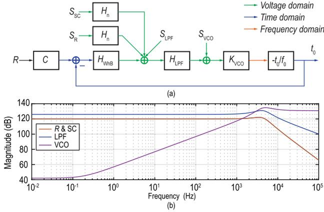
Fig. 6. (a) FLL block diagram and (b) NTFs of the different blocks.
