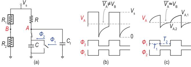
Fig. 3. (a) Schematic of an SC-based WhB and transient waveforms (not to scale) when  $f_0 = 1/RC$  with (b)  $C_f = 0$  and (c)  $C_f \gg C$ .
