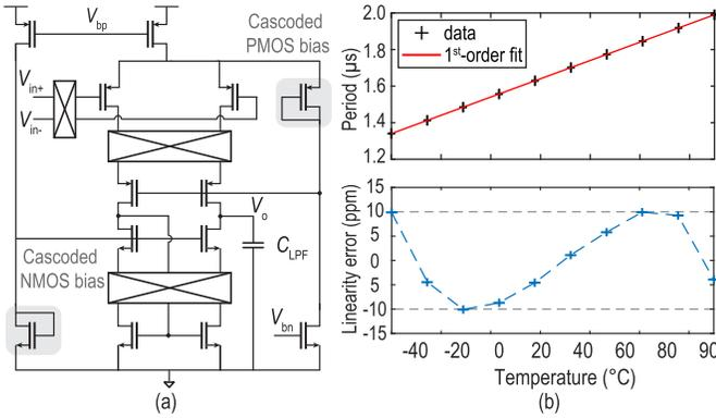
Fig. 8. (a) Schematic of the active low-pass filter and (b) simulated FLL transfer curve and linearity error.
