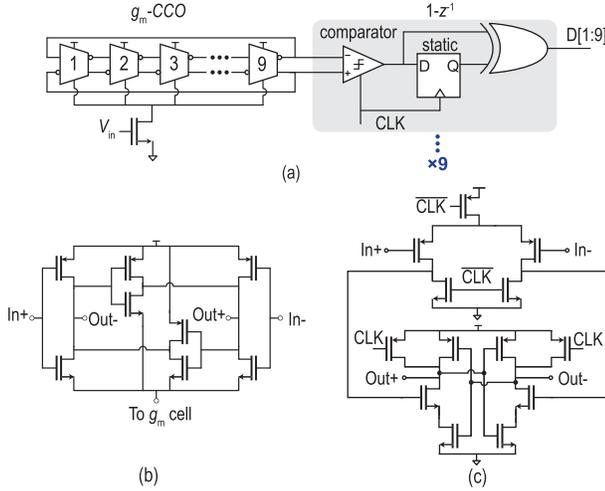
Fig. 10. Schematic of the (a) VCO and TDC, (b) delay cell, and (c) latch.
