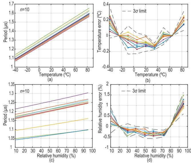
Fig. 16. Measured (a) temperature transfer curve, (b) temperature error, (c) RH transfer curve, and (d) RH error.
