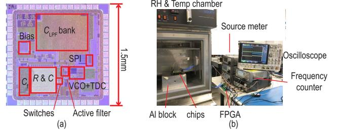
Fig. 11. Photograph of (a) annotated die and (b) measurement setup.
