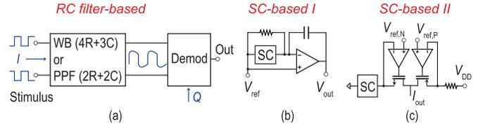
Fig. 2. Examples of prior work that could be used for  $R&C$  sensing, based on (a)  $RC$  filter, (b) SC integrator, and (c) SC resistor and LDO.
