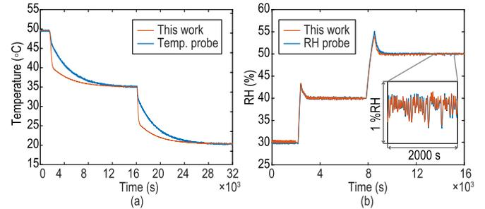
Fig. 15. Measured step response when (a) temperature and (b) RH are changed.
