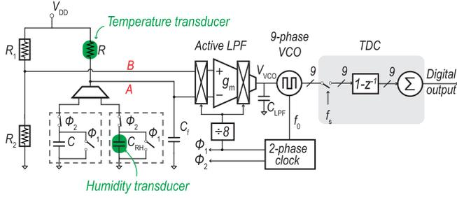
Fig. 5. System schematic of the RH/temp sensor using an RCDC.
