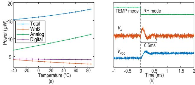
Fig. 12. Measured (a) power versus temperature and (b) transient waveforms during mode switching.
