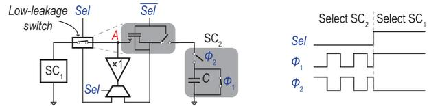
Fig. 7. Schematic and timing of the high-isolation multiplexer scheme.
