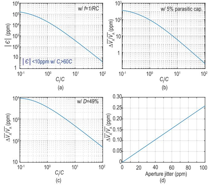
Fig. 4. Simulated (a)  $|\epsilon|$  versus  $C_f/C$ , (b) WhB output change versus  $C_f/C$  with 5% parasitic capacitance, (c) WhB output change versus  $C_f/C$  with 49% duty cycle, and (d) WhB output with a clock phase error.
