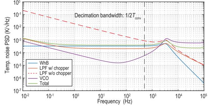
Fig. 9. Simulated FLL noise PSD referred to the temperature input.
