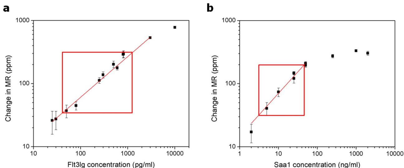
**Figure 2** | Standard curves measured on magneto-nanosensor chips for mouse (a) Flt3lg and (b) Saa1. Red boxes indicate the ranges of magneto-nanosensor chip signal and biomarker concentration used in the assays performed in this work. Error bars are  $\pm 1$  standard deviation.
