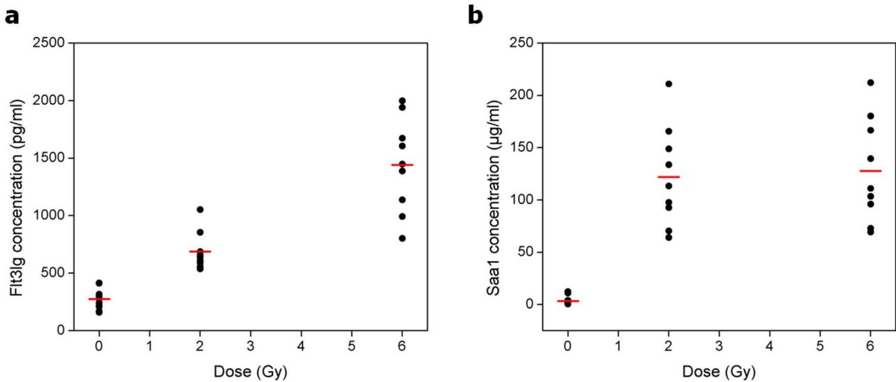
**Figure 4** | Radiation dose response behaviour of mouse (a) Flt3lg and (b) Saa1 measured using magneto-nanosensor biochips for 0, 2, and 6 Gy irradiated C57BL/6J mice at 24 hours post-irradiation. Red bars indicate average values, and each black dot represents one animal.
