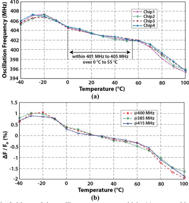
Fig. 5. Measured ring oscillator temperature sensitivity (a) across multiple chips and (b) across multiple DCO modes.
