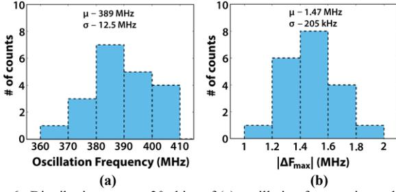
Fig. 6. Distributions across 20 chips of (a) oscillation frequencies and (b) maximum frequency deviation over temperature.
