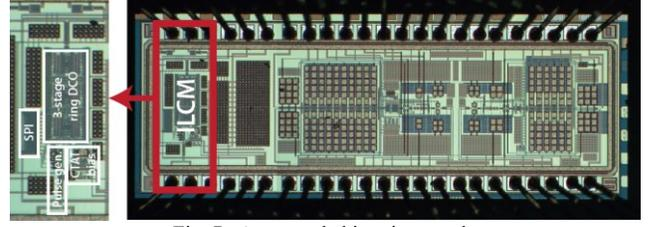
Fig. 7. Annotated chip micrograph.
